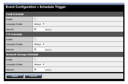
You can separately configure the schedule for trigger function of the camera by **Email**, **FTP**, or **Network Storage**. Select the **Enable** option on each item, and then select a **Schedule Profile** from the pull-down list and set the **Interval** time.
